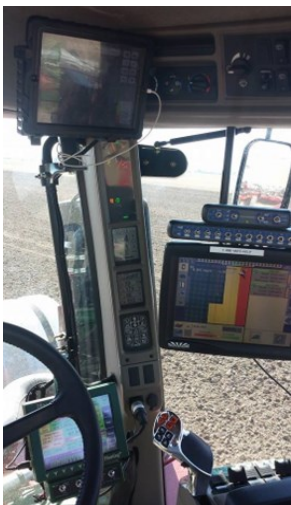
Inside view of the planting tractor. 3 screens run & monitor the tractor and planter.
