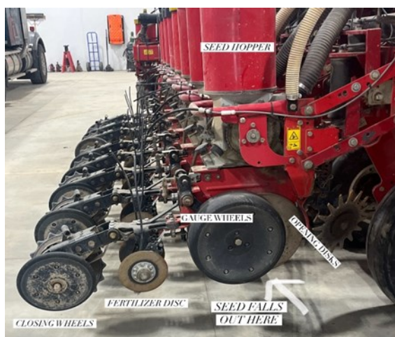
A row unit of a planter. The opening discs open a seed trench, seeds fall individually in a row between the gauge wheels that control the seed depth, fertilizer discs apply fertilizer (plant food) and the closing wheels close the seed trench and cover the row with soil.
